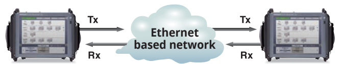
Running Service Activation Test in local - remote configuration using two MT1100A testers
