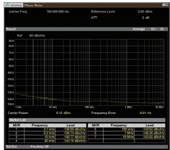
Phase Noise Measurement Low Phase Noise Performance MS2840A-066 On 150 MHz Measurement Frequency, Preamp Off
