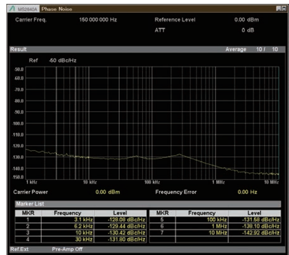
Phase Noise Measurement Low Phase Noise Performance MS2840A-066 Off 150 MHz Measurement Frequency, Preamp Off
